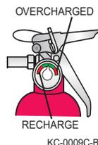
All fire extinguishers used on marine boats must be classified to extinguish type B fires (gasoline, oil or grease). The size and number of required fire extinguishers depend on the size of the boat. The two type B fire extinguishers commonly used are B-I and B-II. Type B fire extinguishers are classified by the different extinguishing compound amounts used in each.
