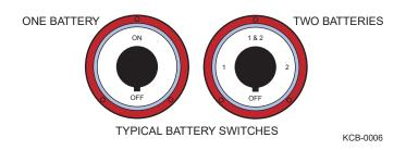
OFF Position - Neither of the batteries are connected to the engine's starting or charging systems. The switch should be in the OFF position when the boat is not being used to ensure that the batteries do not lose their charge. The switch should also be in the OFF position when an external battery charger is being used to charge the battery(s) to avoid possible damage to the electronic components on the engine or in the boat.
