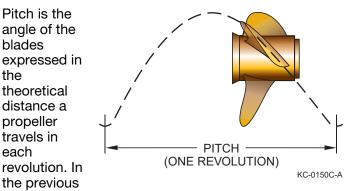
example, the pitch is 19, which means that each revolution of the propeller pushes the boat 19 inches (483 mm) through the water.
