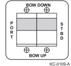
adjust the boat's trim angle and help compensate for uneven weight distribution, listing, water conditions and other factors that contribute to planing inefficiency.
