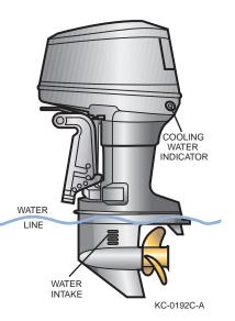
debris which could obstruct water flow into the engine. A continuous discharge of water from the cooling water check port while the engine is running is a visual indication that the engine's cooling system is operating properly.
