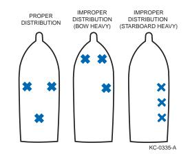
WARNING Sinking Hazard: NEVER exceed the USCG certified maximum capacities under any circumstances. Exceeding the limitations stated on the capacity plate can cause the boat to sink or the passengers and/or operator to drown, resulting in death or serious injury.
