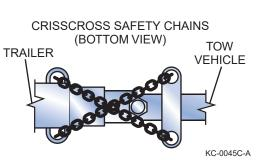
vehicle when underway. Connect the chains to the vehicle's hitch or frame and crisscross the chains under the trailer tongue to prevent the tongue from dropping to the road if the trailer separates from the hitch ball. Rig the chains as tight as possible with enough slack to permit full-free turning. Safety chains must be rated at the same or greater weight capacity as the trailer's GVWR.
