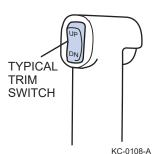
propeller to adjust trim (the planing, and running angle of the boat while underway).
