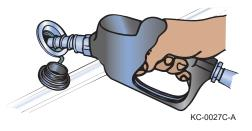
either a shutoff valve or antisiphon valve. The shutoff valve requires you to manually turn the fuel valve, while the antisiphon valve operates automatically. Because gasoline fumes are heavier than air, they will sink to the lowest part of your boat, such as the bilge. Always evacuate fumes with the bilge blower (if equipped) before attempting to start the engine.
