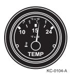
Check the gauge immediately after starting the engine. If the temperature gauge is high, STOP the engine immediately and see the Engine Operator's Manual for corrective action.
