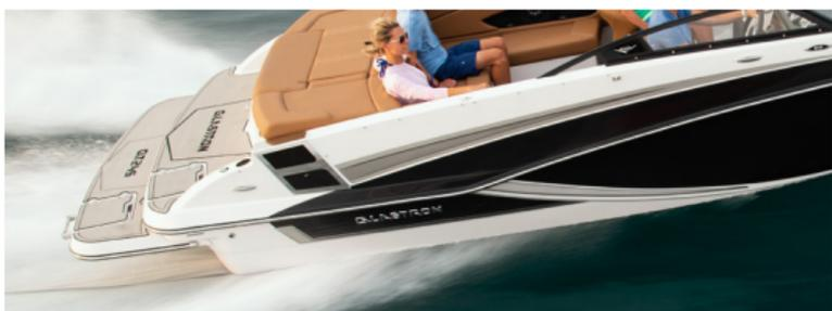
Under power, the SSV hull's wide reverse chines create a "bank" of water for added lift and precise, stable turning. Boats without them have a flatter running surface that results in a more jarring ride with a tendency to slide in turns. On most boat hulls, the chines diminish in the forward half of the hull. In comparison, the SSV hull's wide chines extend far forward. These extended chines reduce rocking from side-to-side and front-to-back by acting as sponsons when the boat is at rest.
