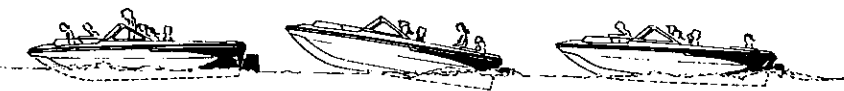
INCORRECT Overload forward Causes boat to "plow" INCORRECT Overload aft Causes boat to "squat" CORRECT Gives maximum performance
