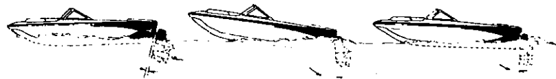
INCORRECT Causes boat to "plow" INCORRECT Causes boat to "squat" or porpoise CORRECT Gives maximum performance
